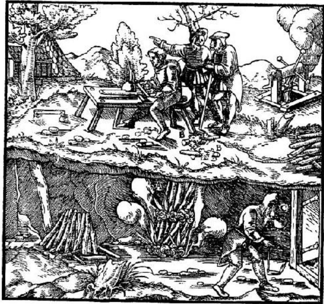
Figure 13: Fire setting, ventilation door.
