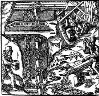
Figure 52: Treadmill driven bucket chain, treadmill (A), axle-tree, double chain (B), a single chain link (D), buckets (E), brackets to fix the buckets to the chain (F,G).
