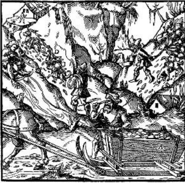
Figure 36: Horse sled (A), sled (B), dogs with pack saddles (D), bellows attached to a rope (E).
