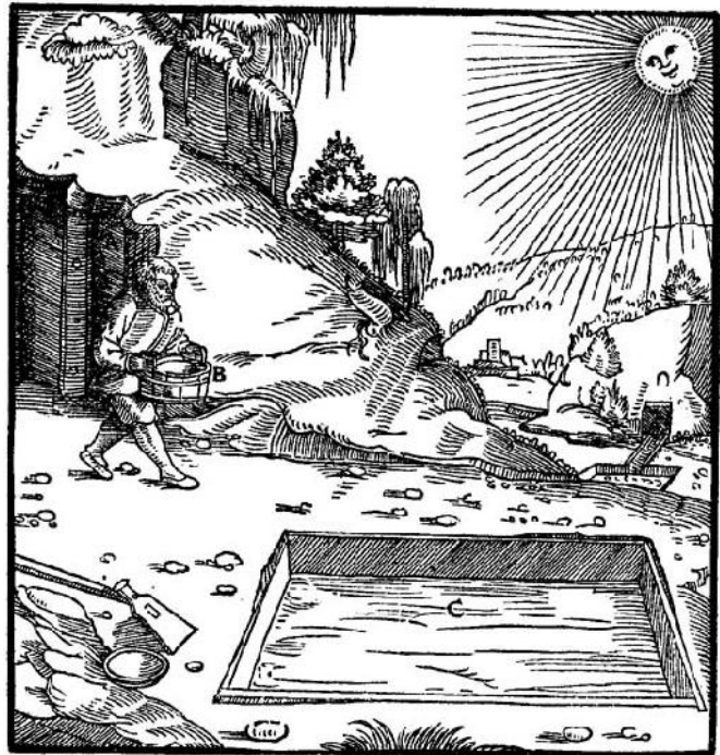
Figure 23: Winning vitriol by evaporation of mine water.
