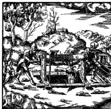
Figure 46: Double acting hasp – pit bank (ABCD) hasp supports (E), iron bearing (F), winch beam (G), crank (K), rope (L), rope hook (M), hoisting bucket (N).
