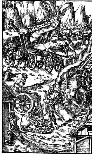
Figure 37: Hoses with pack saddles (A), chute (B, C), single-wheeled cart (D), double-wheeled cart (E), track (F), wagon (G), foreman, noting the number of loads on a counter (K), ore bins (L).
