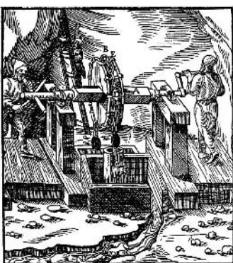
Figure 53: Chain-and-leather-ball scoop – beam (A), chain drum (B), chain (C), stuffed leather balls (D), brackets (E).
