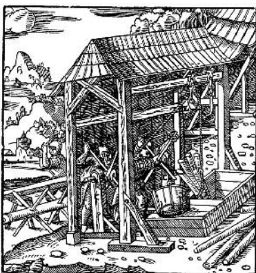
Figure 45: Simple hasp - winch beam (A), crossbars (B), supports (C), haulage rope (D), angle pulley (E), mine timber being brought into the mine (F).
