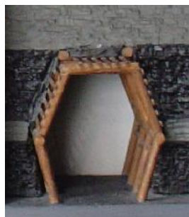
Figure 32: Jointed timbering with parallel khûzan/jarinese roof traversals.
