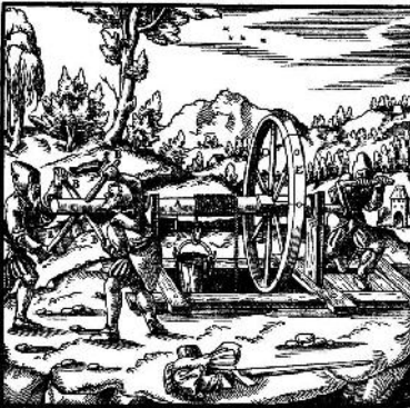
Figure 39: Double acting hasp with flywheel - winch beam (A), crosswise handles (B), crank (C), flying wheel (D, E).
