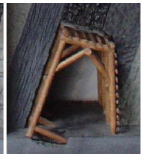
Figure 30: Combined timbering with roof traversal.
